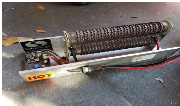
A resistor pack is used during burn testing.
