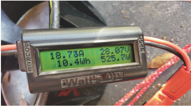
A "WattsUp"® (or other) watt meter can measure battery health.
